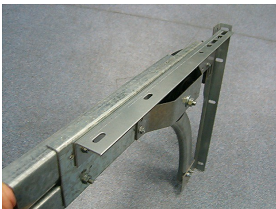
Figure 4 – Low Head Room Rear Track Assembly (Top Horizontal Track not shown in top LH photo). Support angle is added to provide additional support to junction plate, but requires 2 @ Ø7 holes to be drilled (as shown by red circles in bottom RH photo) through support angle to allow fixings to be fitted.
